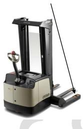
weight of truck balances the load carried on forks
